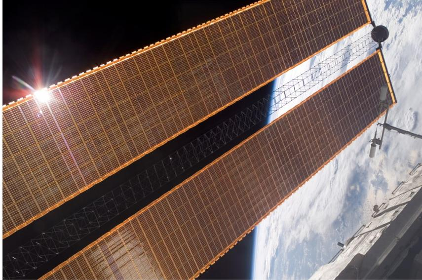
The amount of power generated by each SAW depends on its orientation with respect to the sun and on any shadows on the solar collectors. Code to calculate the power generated at a specific orientation will be provided for the use by contestants in the off-line tester/visualizer.
